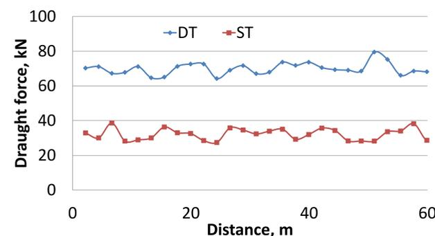
Figure 4. Draught force (kN) requirements in tillage
