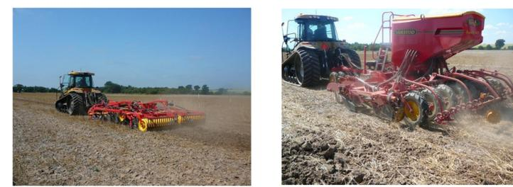
Figure 2. Combination tiller (a) and direct drill (b)
