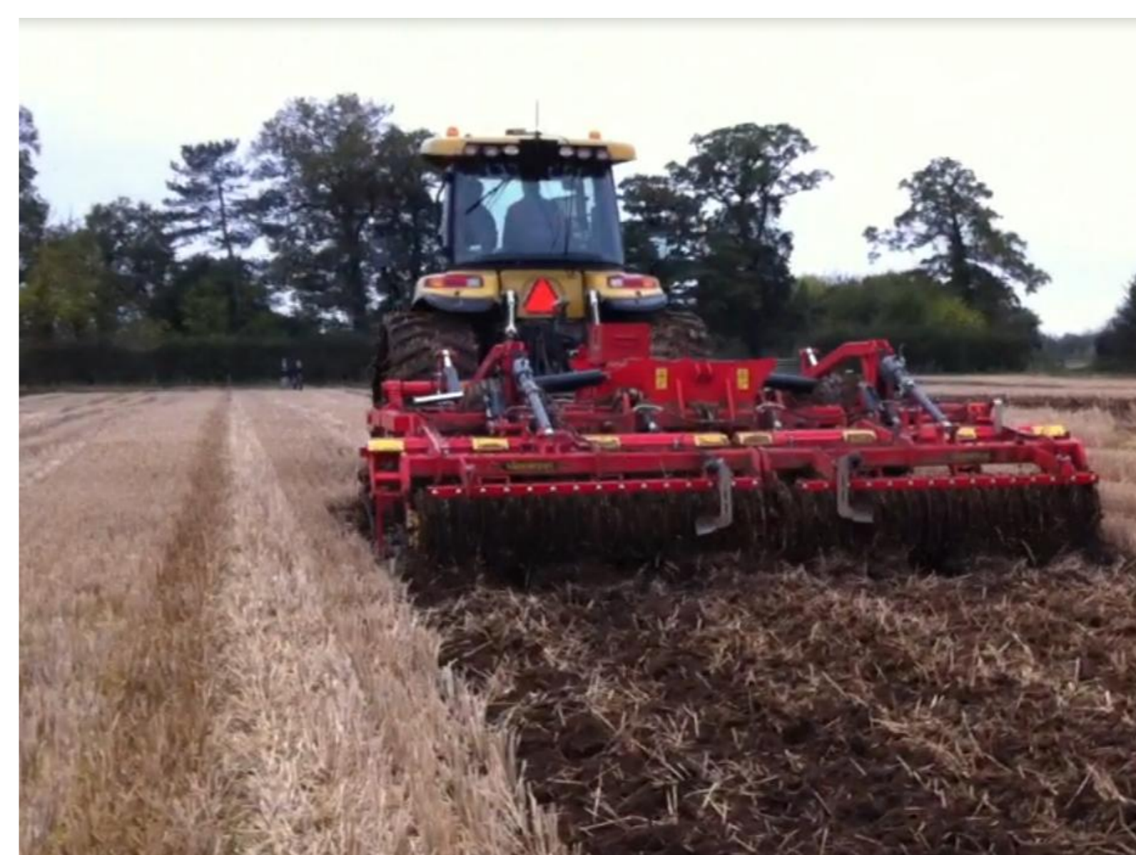
Vaderstad TopDown cultivator for deep and shallow plots. Vaderstad Rapid for drilling all plots.
