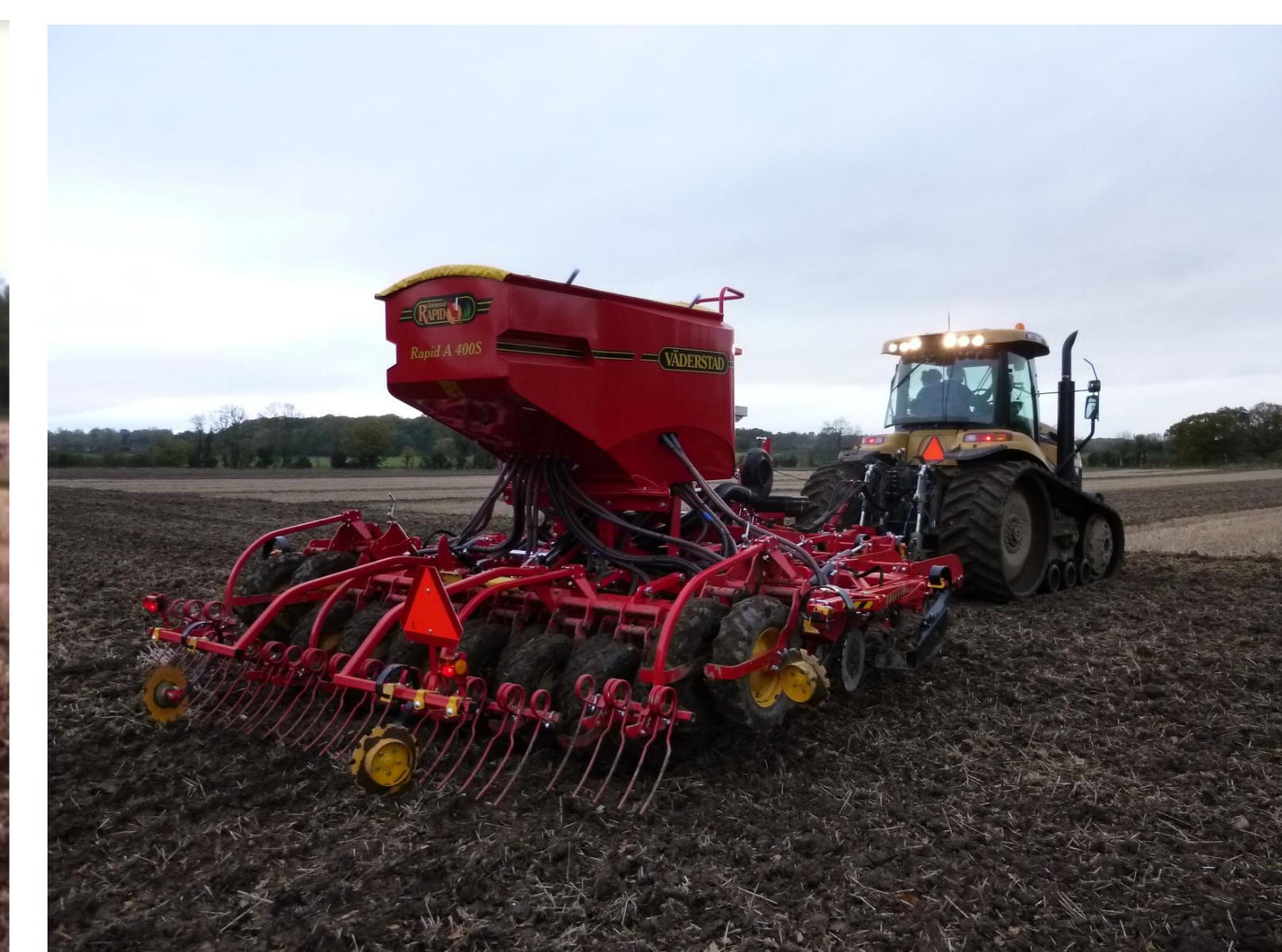
Vaderstad TopDown cultivator for deep and shallow plots. Vaderstad Rapid for drilling all plots.
