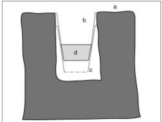
Figure 1. Cross-section through a pitfall trap: a) ground surface; b) pitfall trap (coffee cup); c) liner cup with perforated base; d) trapping liquid (water and detergent).
