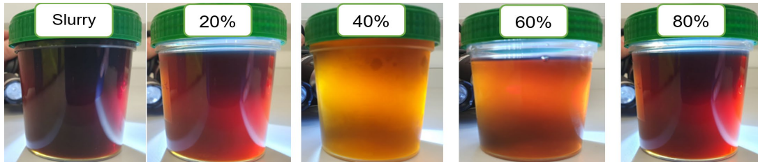
Figure 1 – Reverse osmosis concentrated, nutrient-rich fraction samples produced from cattle slurry (from left to right: original cattle slurry (untreated), 20%, 40%, 60% and 80% volume of water fraction removed from the cattle slurry using reverse osmosis)
