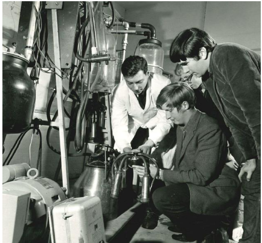
Here we have an image displaying a workshop demonstration of a milking machine unit and plant in January 1969, this image was taken as part of a series of photographs covering the activities at agricultural colleges and institutes in England and Wales.
