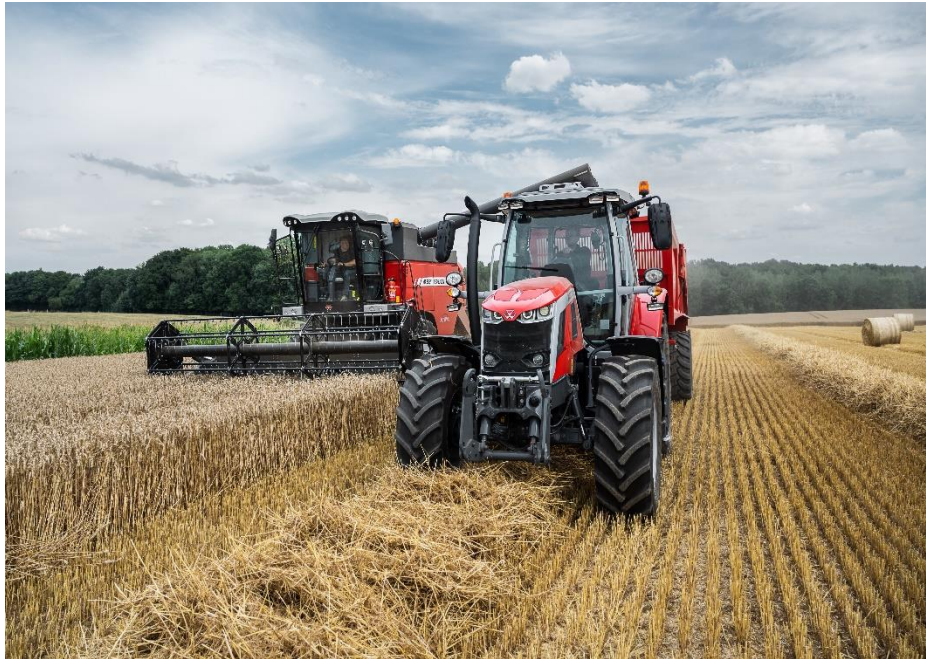
Figure 13. A combine harvester and chaser wagon remaining on track in a CTF system.
