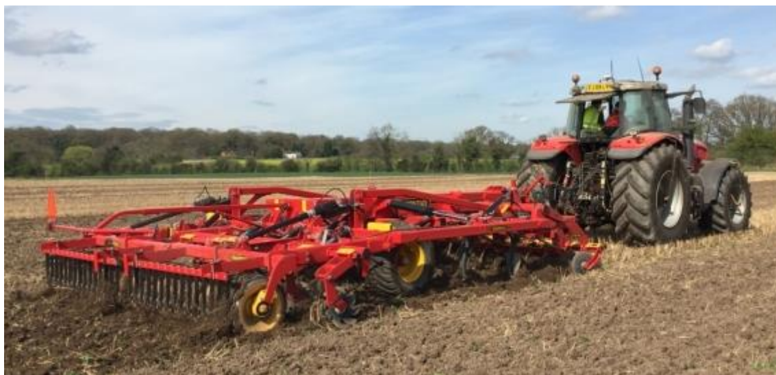
Figure 2. Massey Ferguson 8480 tractor with a 4 m wide Väderstad Topdown multipurpose cultivator at the experimental site
