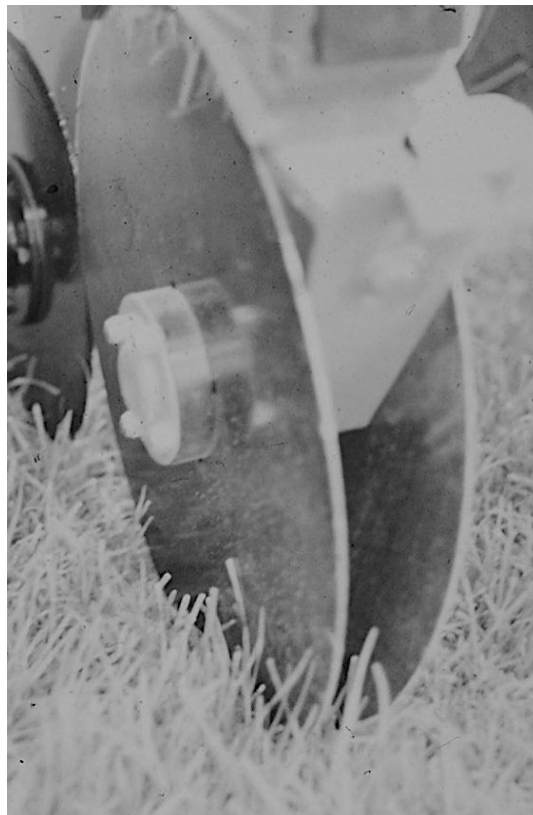
Figure 5. An early double disc type coulters. (Courtesy: Spoor)
