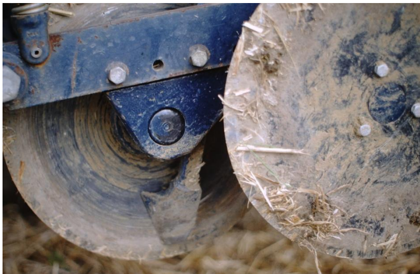
Figure 11. Modified Moore 'Unidrill'. Showing seed placement coulter. (Courtesy: Spoor)
