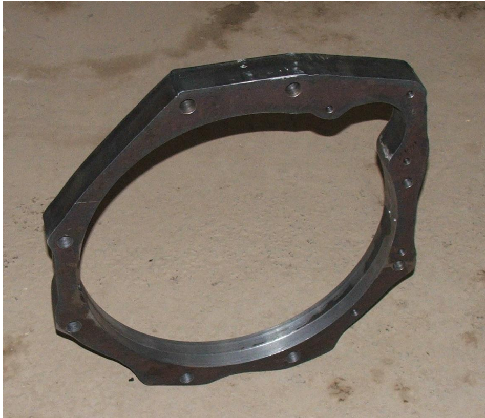
Figure 3.3: The 50mm steel plate used to extend the tractor (Source, author)
