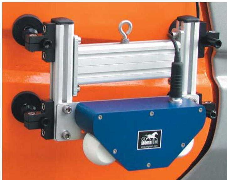
Figure 3.10: The Pegassem GSS20 dual head microwave speed sensor. (Source, Pegassem 2005)
